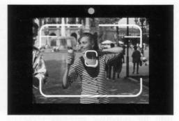
Holding the camera to the eye, point it at the subject so that the main parts, i. e. those that must be in focus, are inside the autofocus frame. Now press the shutter release button lightly, (tp pressure point). The green confirmation symbol appears in the viewfinder to show that the focus reading has been stored.
