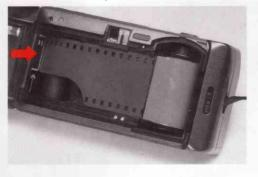
4. Close the camera back and switch on the camera. The film advances automatically to the first frame. The camera is ready for the first exposure when the frame counter is at "1". If the frame counter displays "0", the film is not loaded properly. Reopen the camera back, remove the film and re-insert it as decribed under 2-4 above.
