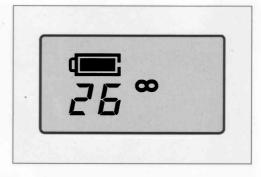
Note: To take several pictures consecutively in the infinity setting, the mode control button must be held down after pressing it 3 times for approximately 3 seconds until "\infty" flashes. To cancel and return to "AUTO", press the mode control button once more. When the camera is switched off and subsequently switched on again, it is automatically set to the automatic program mode "AUTO".
