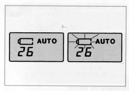
If the symbol  $\square$  flashes, or if no display is shown, it could be that the battery contacts are oxidized or soiled. They can be cleaned with a clean, dry, lint-free cloth. If the battery is partly discharged, the symbol  $\square$  may also appear after a series of exposures in close succession. Before further exposures, pause briefly for the battery to recover.
